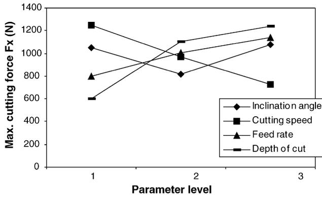
Fig. 4. Mean effect plots for cutting forces  $F_x$ .
