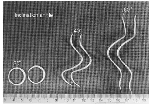
Fig. 7. Photographs of chips produced during self-propelled round insert face-milling operation at different inclination angles. Feed rate 200 mm/min, depth of cut 0.5 mm.
