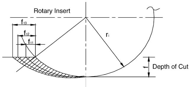
Fig. 8. Model to demonstrate the effect of feed rate the hip cross-section area.
