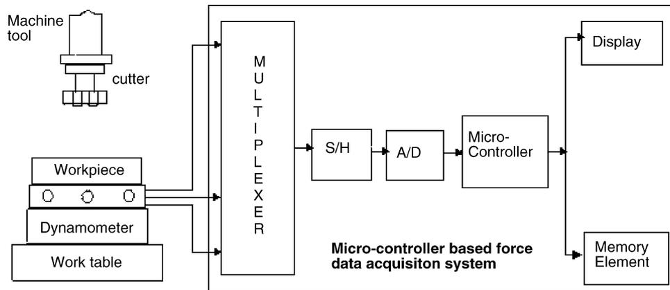
Fig. 2. Multi-channel analog multiplexed force data acquisition system.
