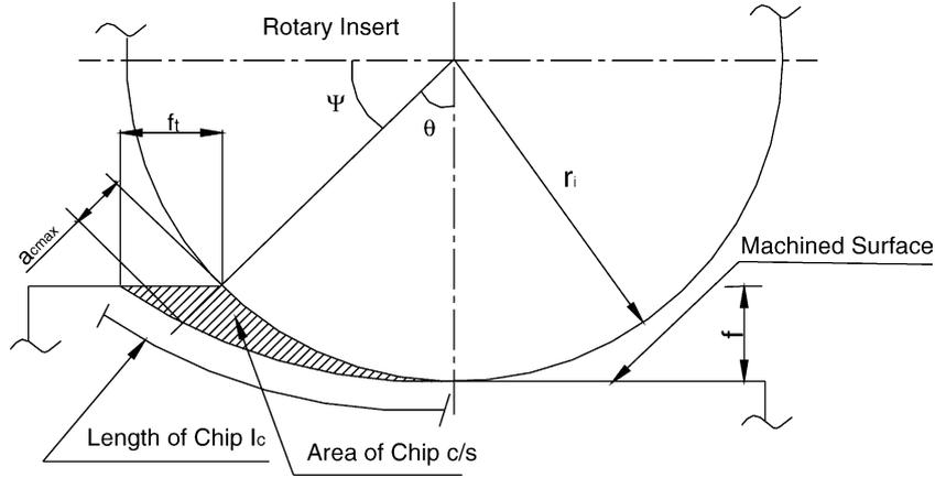
Fig. 10. Geometry of chip in rotary inserts.
