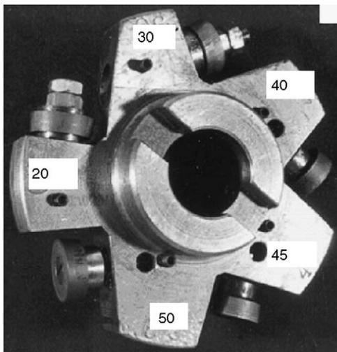
Fig. 1. Self-propelled face-milling cutter with round inserts at various inclination angles [9].
