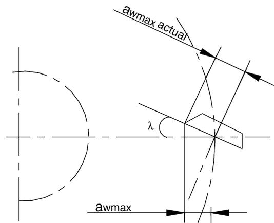
Fig. 11. Effect of insert inclination angle on self-propelled face-milling.
