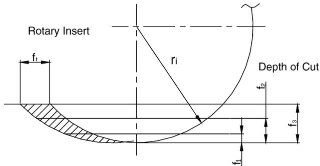
Fig. 9. Model to demonstrate the effect of depth of cut on the chip cross-section area.
